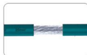
Piercing effect of wire core
