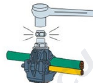
6. Screw the nut continually until the top part is cracked and dropped down.
